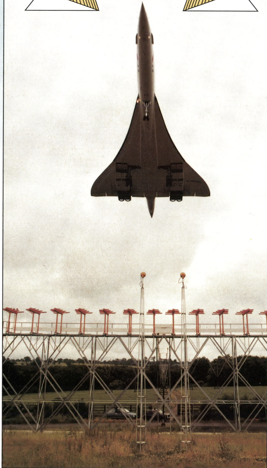
Left: Concorde flying over a Racal Avionics Instrument Landing System Localiser Aerial at Luton Airport.
